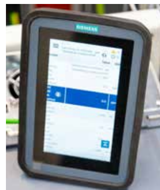
The SINAMICS Smart Drive Interface enables effortless operation, monitoring, maintenance, and on-site service with plain-text messages
