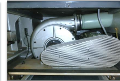
Standard configuration of GD121 with internal fan for vacuum chamber
