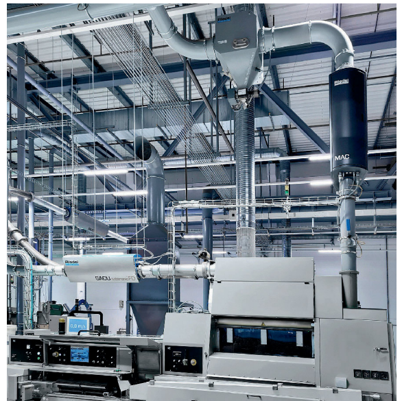
Cigarette makers equipped with Riedel’s technologies like MAC (Maker Airflow Control), SACU tobtronic® and TIRS (Tobacco Shorts Recovery)
